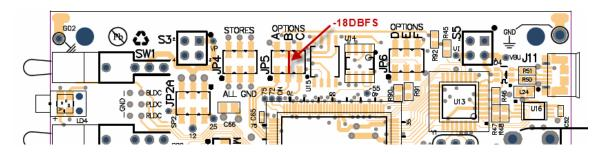
The Voice ID factory default is set for 1 second announcements and 14 seconds of tones which yield a 15 second cycle time. There is a jumper selection to cut the voice announcement time in half, basically by removing the word "Channel" from the voice tags. This yields a cycle time of 7.5 seconds. After removing the case and battery board, locate the options header JP5, and move the suitcase jumper to short pins at the "C" position for 0.5 second voice IDs.
